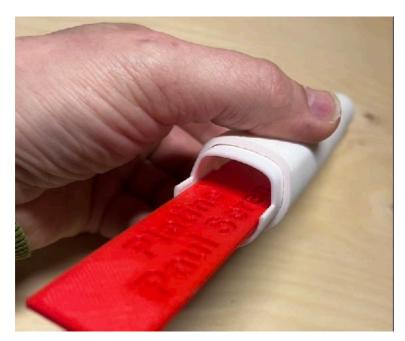
The Insertion of the board must be by inserting the adhesive Adapter. This is important, otherwise the board will be tilted and not in the right position.
